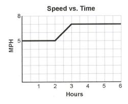
On a speed-time graph, distance is equal to the area between the baseline and the plotted line. You know that the area of a rectangle is found with the equation:  $A = L \times W$ . Similarly, multiplying the speed from the *y*-axis by the time on the *x*-axis produces distance. Notice how the labels cancel to produce miles:
